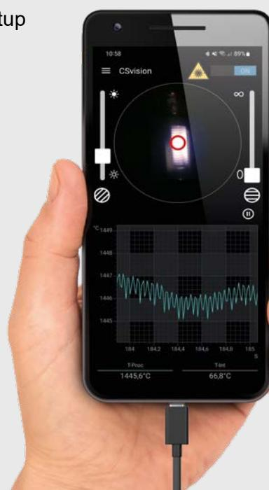
The innovative two-step brightness reduction filter uncovers tiny details: here of a filament.
