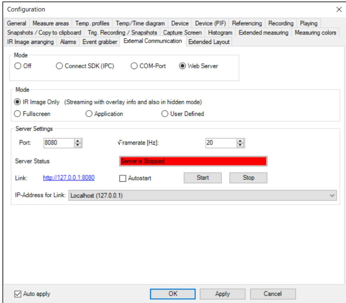
The IR image can be called up via a browser via the link address with the port number.
