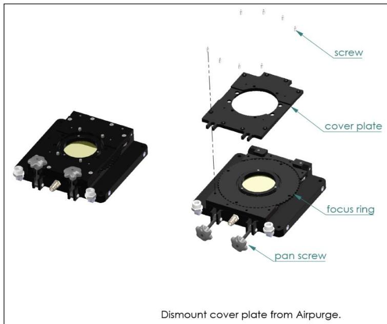
**Figure 51:** Assembly of the laminar air purge
