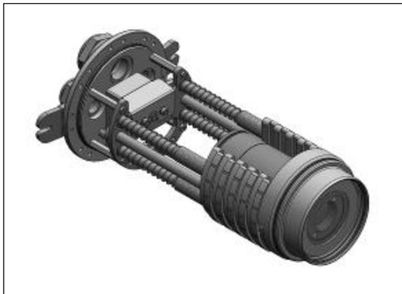
**Figure 33:** Front part with infrared thermometer
